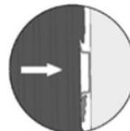
3. Push the upper edge of Lock parallel to the wall
