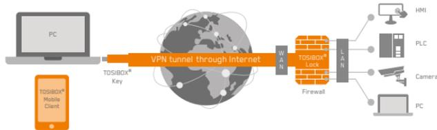
With its factory default settings, the Lock is connected to the Internet via its WAN port or a USB modem which can be connected to the USB port of the Lock. In this mode, the Lock creates its own protected local network for the connected devices. In this configuration, only devices that are connected to the Lock by cable or via WLAN access point are accessible with the Key.
