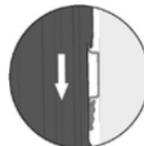
4. Slide the Lock down and check that the DIN rail bracket has a firm grip of the DIN rail
