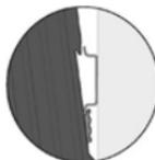
1. Place the DIN-rail bracket slider under the lower edge of the DIN rail.
