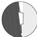
1. Place the DIN-rail bracket slider under the lower edge of the DIN rail.
