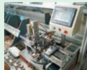
Automatic Rivet Passing, Riveting & Inspection, Screw Back & Inspection and Delay Detection.
