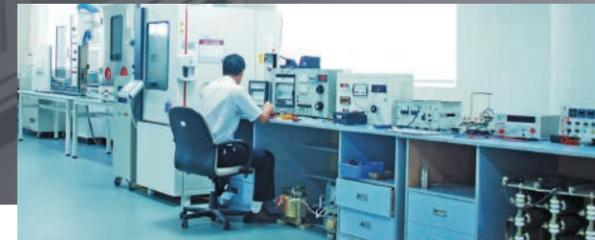
Xenon-lamp weather resistance. Force and travel/conduction angle and travel/resistance and travel tester. Dust proof test IP5X and IP6X. Waterproof test IPX4, IPX5, IPX6 and IPX7. Glow wire apparatus. Tracking index apparatus (test voltage; 100-600V). Agilent Multi-channel temperature tester (34970A). Heraeus drying oven. WV Alternating humidity temperature test chamber (-40~+180°C, 10%-98%). KIKUSUL Withstanding voltage tester. Insulation Resistance tester. Earth continuity tester.
