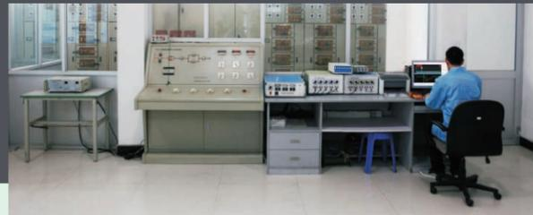
Our Short-Circuit testing laboratory is independent of the endurance test laboratory. We can carry out AC and DC short-circuit test, with a maximum current of 10000A, voltage of 500V and is accredited by American UL and CTDP, German VDE and TUV, Swedish Intertek ETL and SEMKO.
