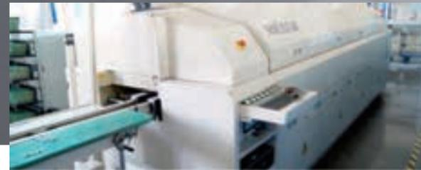
The Electronic Production Workshop is controlled to be Dust-free with an advanced SMT machine, with lead-free reflow soldering. Our wave soldering equipment improves production efficiency and consistency.
