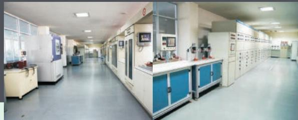
The KEDU electrical switch laboratory is accredited by American UL and CTDP, German VDE and TUV, Swedish Intertek ETL SEMKO. The Laboratory is designed according to UL, VDE, CE and ENEC standards. The maximum test current can reach 2000A and a voltage of 500V, all product tests rated within 300A. Up to 60 switches can be tested at the same time. Products are processed to acquire UL, CUL and CSA (Canada), VDE (German), TUV, CE and ENEC and Swedish SEMKO Certification.
