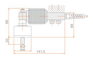
Protects load cell against lateral loads. Used in accurate and vibrating weighing systems.
