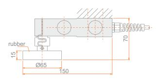
Protects load cell against lateral loads. Used in platform scales. Enables leveling
