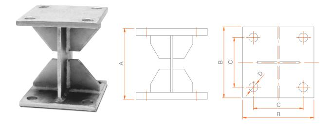
Esit ET flexible conveyor is an economic solution for weighing of liquid or gas tanks, which do not require an accuracy of more than 1/1000. A combination of one load cell and two flexible conveyors is suitable for tanks connected at three points whereas for tanks connected at four points, this combination shall include two load cells and two flexible conveyors. The flexible conveyor can be used with Esit TM, EL and ELT mounting kits.
