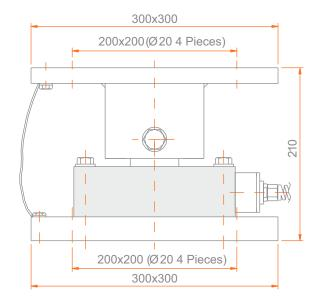
Avoids toppling or displacement of the load with the ground fixing system Corrects off-center loads
