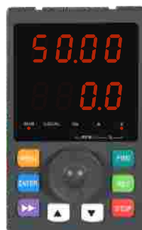
Figura C Running status, showing the operating status parameters
