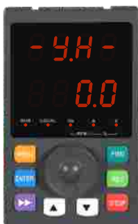
Figura A Power on to initialize the display dynamic picture
