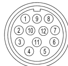
HA connector (12 pin) M23 CCW Hummel 7.410.000000 - 7.002.912.603 solder side view FV
