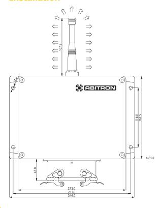
The antenna has to point vertically upwards!
